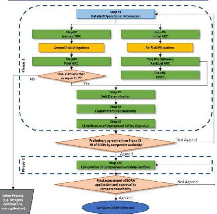
This flowchart outlines the Specific Operations Risk Assessment (SORA) process, which is used to evaluate and approve drone operations based on safety risk. Here's a summary of the process:
