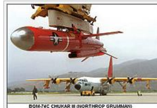
BQM-74C CHUKAR III (NORTHROP GRUMMAN) A BQM-74 Chukar III, turbojet-powered aerial target.
