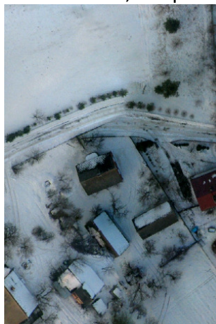
Non-stabilized head, locally reduced overlap led to mismatched road geometry. Pteryx UAV is completely free from those troubles.
